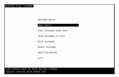
Use the arrow keys to move around the options and hit enter to make a selection. The PROGRAM RADIO and READ RADIO options are used to load or read back the configuration from a transmitter, the configuration can be read from or saved to disc using the LOAD and SAVE options, QUIT exits the program, EDIT PROGRAM and TEST/CALIBRATE lead to further menus:
