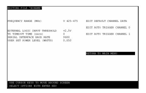
Auto trigger channel 0 is set up for the Pocsag pager.
