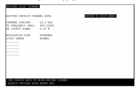
The default channel data has been set for external modulation. The logic sense has been set to normal however this option only affects digital encoders.
