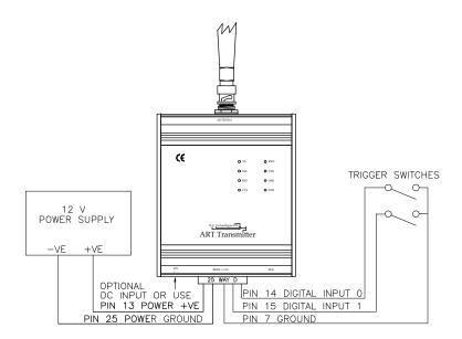
For the purpose of this example we shall say that trigger input 0 is to cause the text message "Alarm zone 23" to be sent to a 1200 baud Pocsag pager with the address 1234567, the pager's frequency is 466.075 MHz. Trigger input 1 is to cause the selcall tone sequence 54321 to be sent to a hand portable radio transceiver on 458.5 MHz, the radio uses the CCIR 70ms tone format. The set-up program would be edited as follows:
