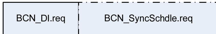
Figure 9-18 – Example of a beacon frame format including the BCN_DI.req message and one additional beacon message (BCN_SyncSchdle.req)
